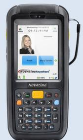
*The portable and rugged NT65M is the ideal hardware solution for a mobile workforce. The certified Wi-Fi and Wireless WAN capabilities provide secure communication for real-time data transfer and up-to-date information, while the IP67 rating ensures complete protection against dust and water damage.*
